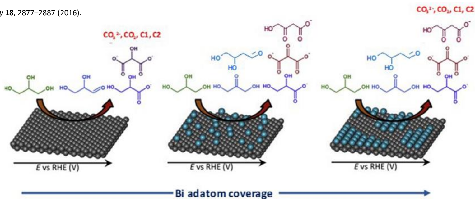
Influence of the coverage of a Pd surface by Bi adatoms on selectivity of glycerol oxidation reaction (Zalinee et al., 2015).
